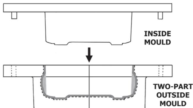
**Fig 5. Making a bellied bowl. During casting, pewter fills the light and dark grey zones. The light grey zone, which is only 2-3mm thick, is then removed on a lathe.**
